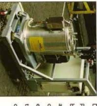
Designed for pilot plant test production and for small batch treatment this reliable and robust machine offers customers the chance to evaluate the behaviour of their product under centrifugation.
